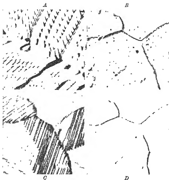
A, SILVER HEATED IN OXYGEN FOR 11 HOURS AT 920° C (×2000). B, SILVER HEATED IN NITROGEN FOR 11 HOURS AT 920° C (×250). C, SAME FIELD AS B, AFTER SUBSEQUENT HEATING IN AIR FOR 1 HOUR AT 920° C (×250). D, SAME FIELD AS B, AFTER FURTHER HEATING IN NITROGEN FOR 11 HOURS AT 920° C (×250)
